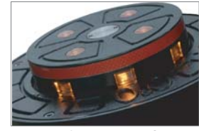
Hat – light consist of 8 LED lights on side and 4 LED above
